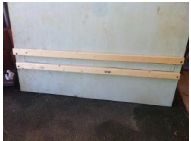
Anchor boards attached to the underside of the door/tabletop
